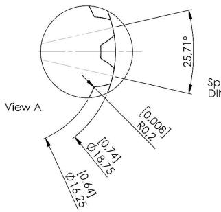
Spline geometry DIN 5480-W19x1,25x30x14x8h
